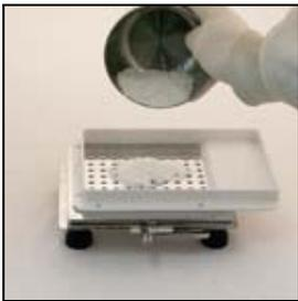
**9.** Place Powder Tray on Filler using locating pins and pour out pre-measured powder.
