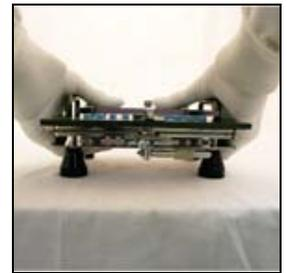
**12.** Place Caps Tray back onto Filler. To lock capsules, push down on Locking Plate with thumbs while pulling up on Lifting Plate with fingers.
