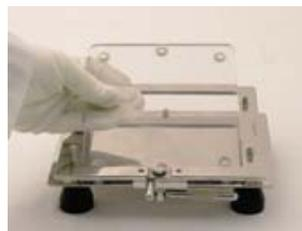
**5.** Lift out the Spacer Plate and replace with the new size Spacer Plate.
