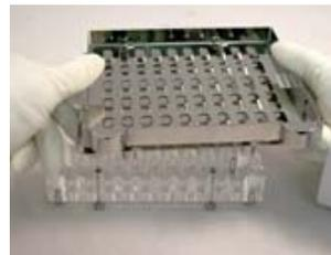
**2.** Align the locating hole in the new size Orienter Change Part with the locating post on the correct size Base. Tighten the 4 hand screws.
