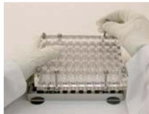
**1.** Turn the Orienter over and remove the 4 hand screws from the Base. Remove the Orienter Change Part.
