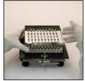
**4.** Push the sliding portion of the Orienter to the left to drop capsules into the Filler.
