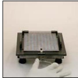
**7.** Close the Filler Locking Plate and slide Locking Clamp to secure. Gently squeeze the Cam Lever toward the post to secure bodies in the Filler.
